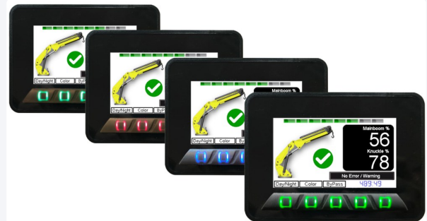
Night mode dims the display and illuminates the buttons. Button LEDs available in four colours
