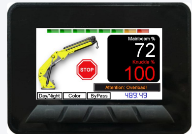
Overload. STOP shown, crane halted
